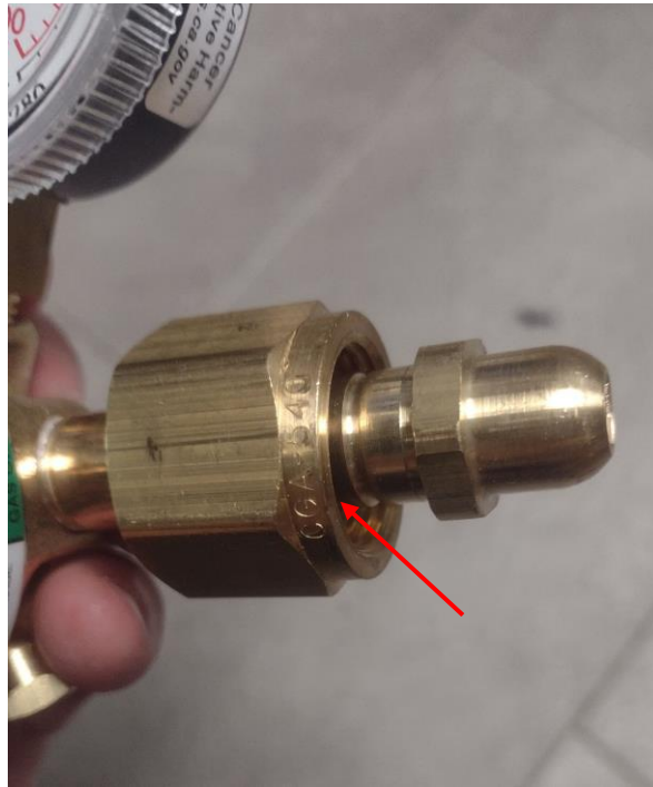
Note the CGA540 markings on the nut
