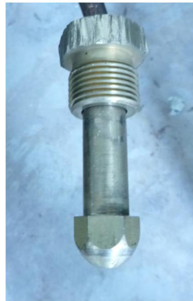
Note there is no rim, and the radius is larger than the French nipple
