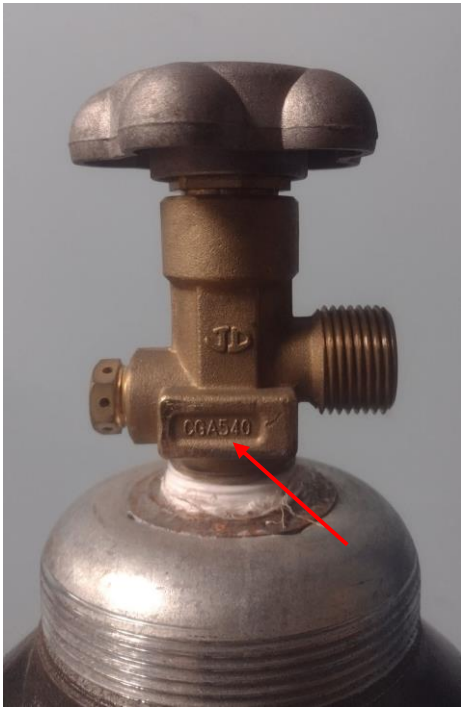
Note the CGA540 markings
