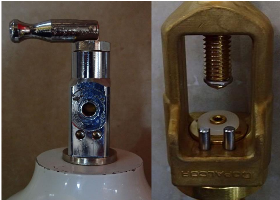
Figure 5: Pin Index Safety System Numbers
