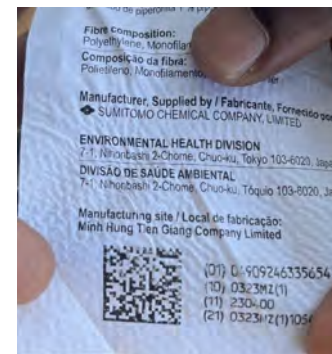
Image of a damaged code (code with net imprint / wrinkled barcode)
